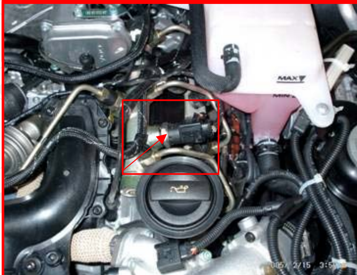
Pressure Transducer Sensor T-cable cable connection engine
