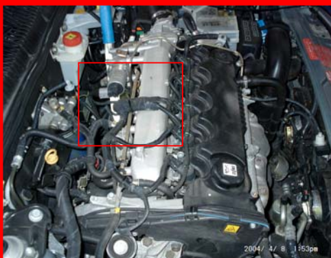
Close up rail pressure sensor III.3
